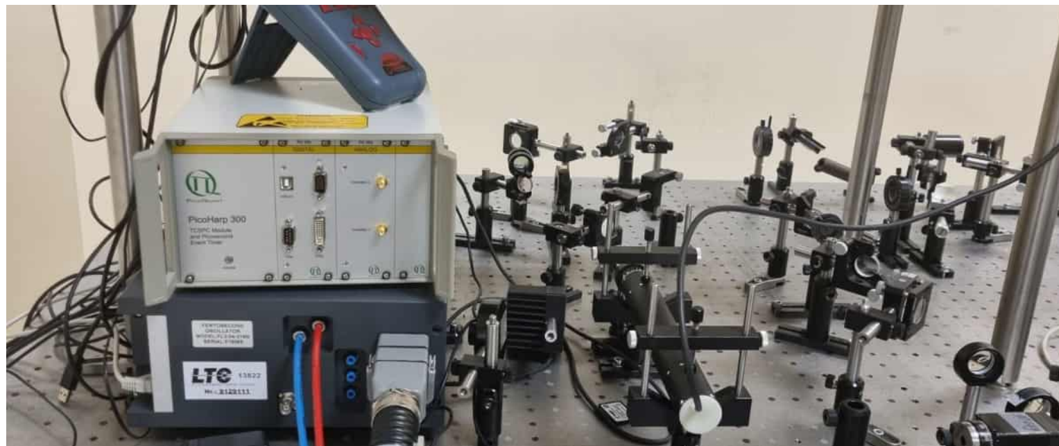
Femtosecond oscillator „Flint“ ( Light Conversion ) and time-correlated single-photon counting module „PicoHarp 300 ( PicoQuant ) used in quantum optics experiments.
